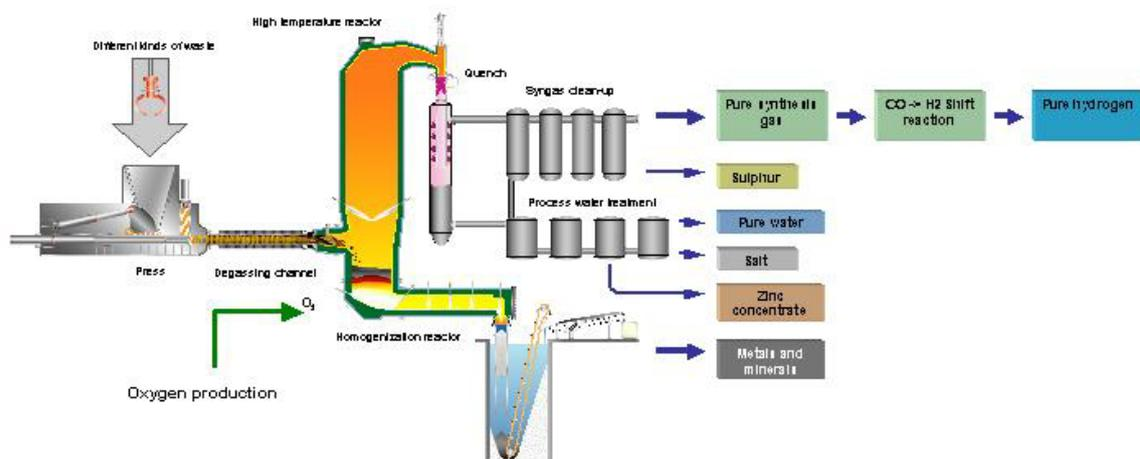
In the Thermoselect process the following materials are produced from 1 ton of waste and app. 520 kg oxygen: 900 kg Synthesis gas, 350 kg cleaned water, 230 kg
